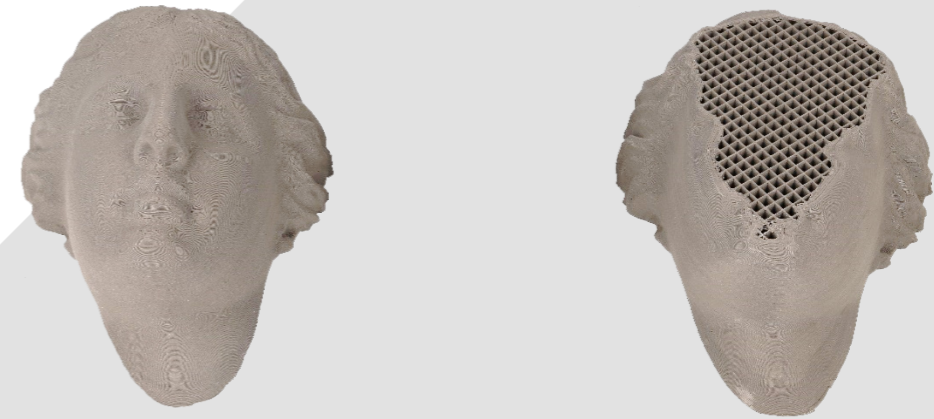
Figure 21: Mass Reduction Using Infill
