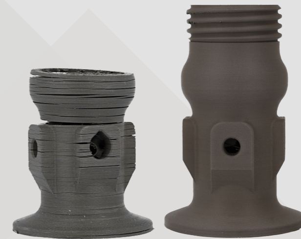
Figure 22: Cooling & Delamination Example
