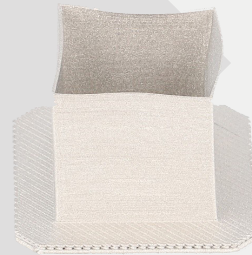
Figure 18: 0.4mm Wall Failure
