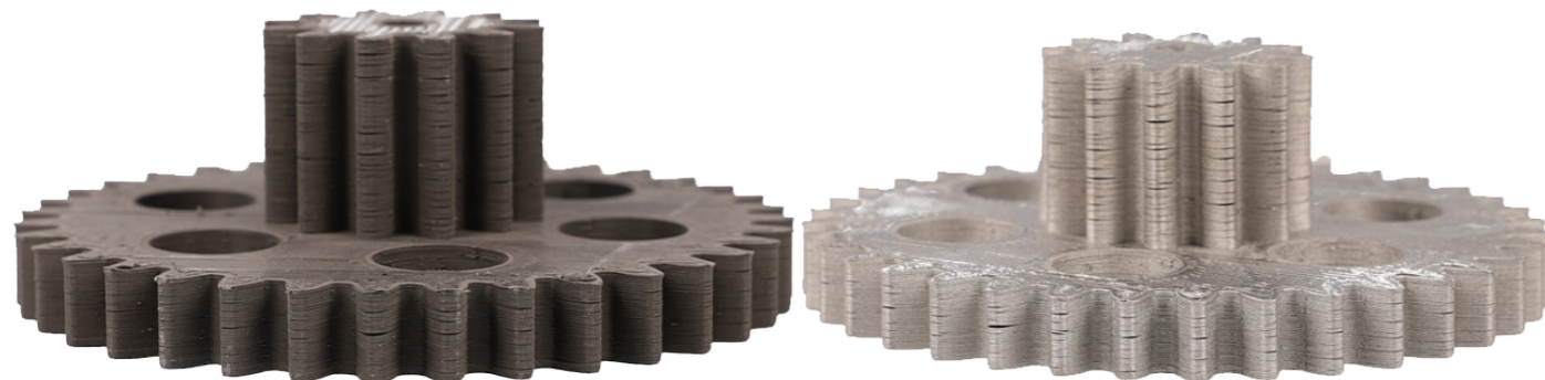
Figure 6: Print Delamination Become Sintered Cracks
