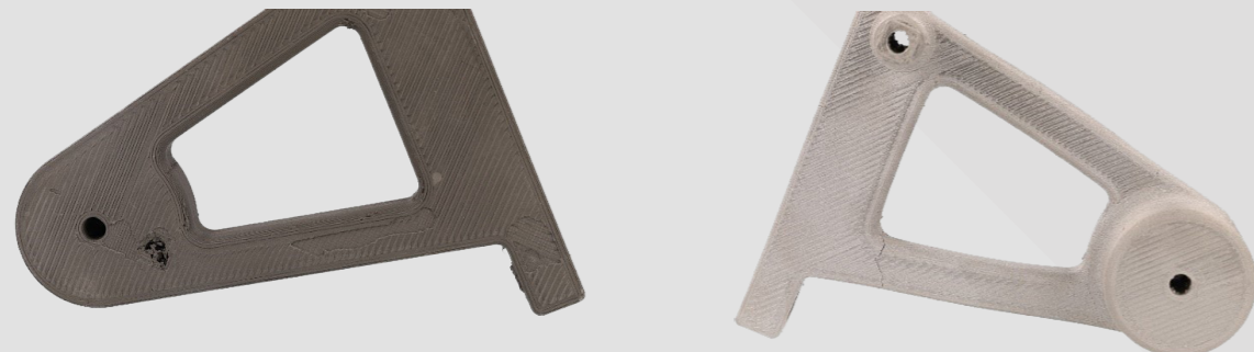
Figure 16: Damaged Bottom Surface and Resulting Top Cracks
