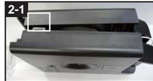
Press the joint of the casing of the filament cartridge gently and open it.
