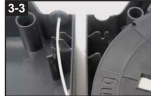
Direct the filament through the guide hole to put out the filament easily.
